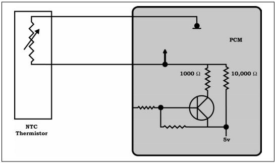
Figure 47 SBEC Dual Range Engine Coolant Temperature Sensor
