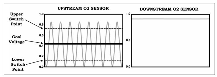
Figure 54 Goal Voltage and Switch Points Shift to Increase Low O<sub>2</sub> Content
