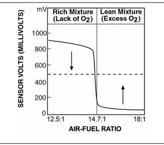
Figure 51 Oxygen Sensor Signal
