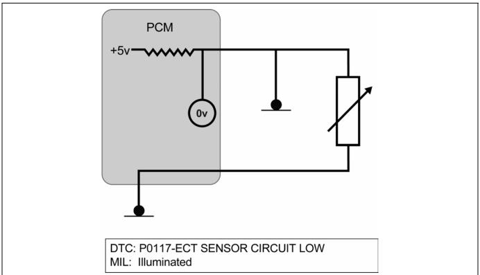
Figure 8 PCM Circuit, Short to Ground
