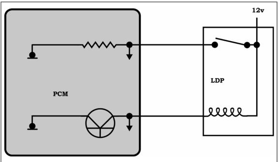
Figure 89 Leak Detection Pump
