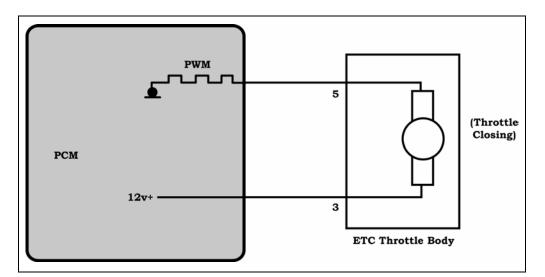
See Figure 97, Page 149 ETC Motor Polarity with Throttle Closing
