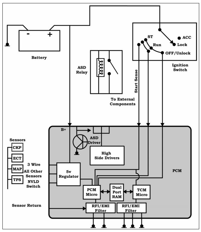
Figure 30 NGC ASD Relay and 5V Regulator (Completed by Student)
