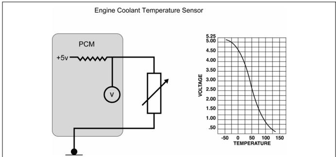
Figure 7 PCM Circuit, Variable Input
