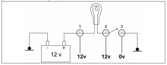
Figure 1 Open Series Circuit
