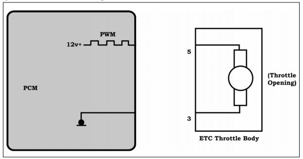
Figure 96 ETC Motor Polarity with Throttle Opening (Completed by Student)
