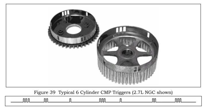
Figure 40 Typical V-6 / Inline 6 CMP Scope Pattern (NGC shown)
