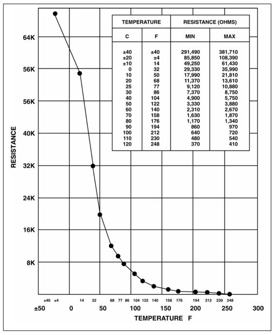
Figure 45 Typical NTC Thermistor Temperature-Resistance Curve
