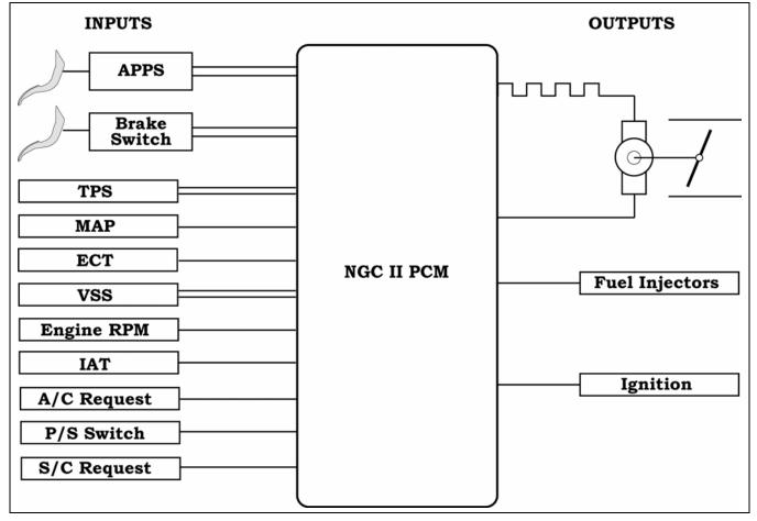
Figure 90 NGC II PCM Inputs and Outputs
