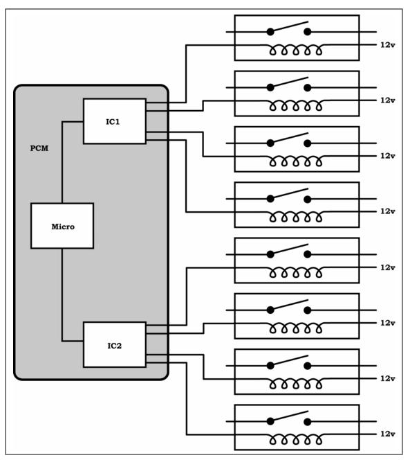
Figure 66 Low Side Output Control
