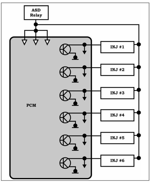
Figure 72 NGC Fuel Injector Control Circuit
