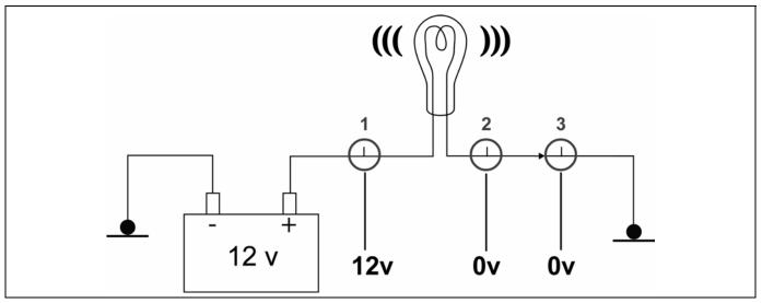
Figure 2 Closed Series Circuit
