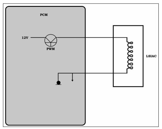
Figure 82 Linear Solenoid Idle Air Control Valve
