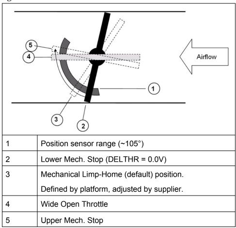
Figure 103 5.7L ETC Throttle Plate Stops
