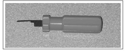
Figure 20 Miller #6932 Pin Removal Tool - SBEC
