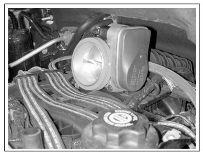
Figure 95 5.7L ETC Throttle Body
