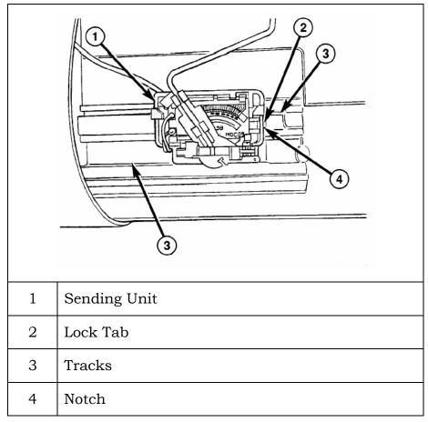
Figure 13 Typical Fuel Level Sending Unit
