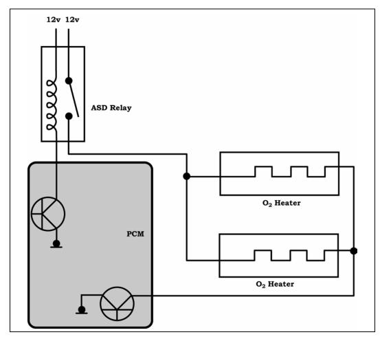
Figure 57 Oxygen Sensor Heater Element - ASD Power / PWM Ground
