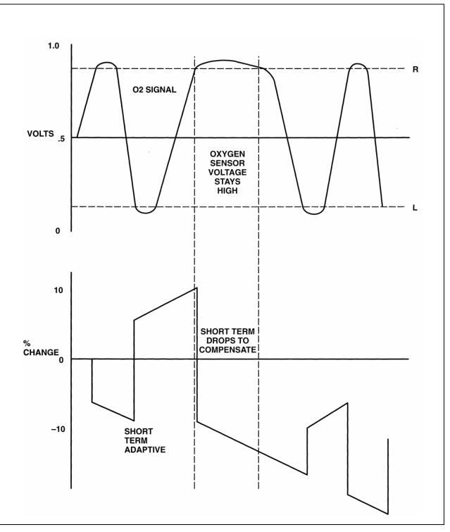
Figure 59 Short Term Adaptive vs. O2 Sensor Voltage
