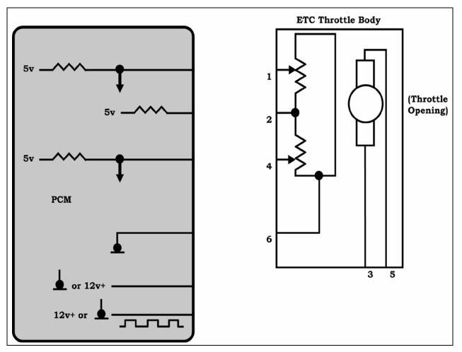
See Figure 100, Page 152 Electronic Throttle Control Circuit
