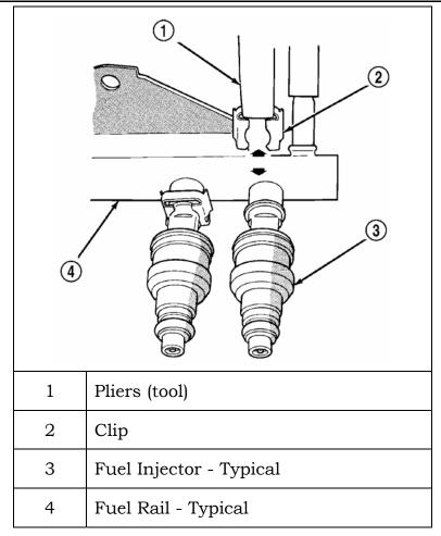
Figure 73 Fuel Injector Clips
