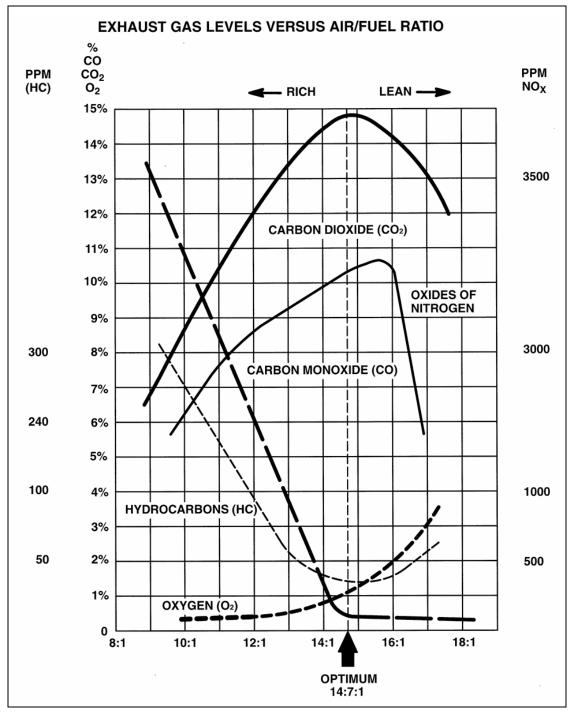
Figure 33 Exhaust Emissions vs. Air/Fuel Ratio
