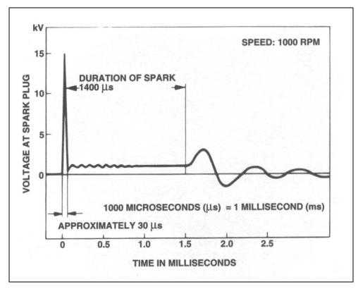
Figure 75 Secondary Ignition Voltages
