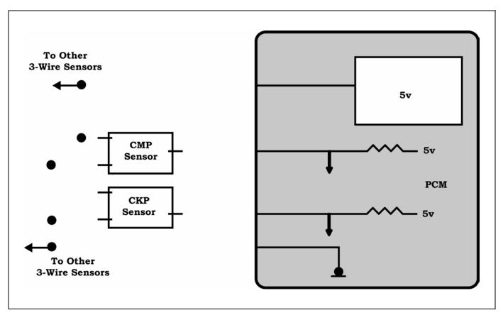
Figure 36 CMP and CKP Sensors (Completed by Student)
