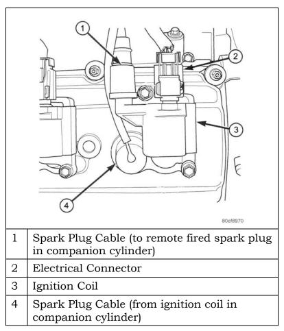
Figure 80 5.7L Ignition Coil Installation
