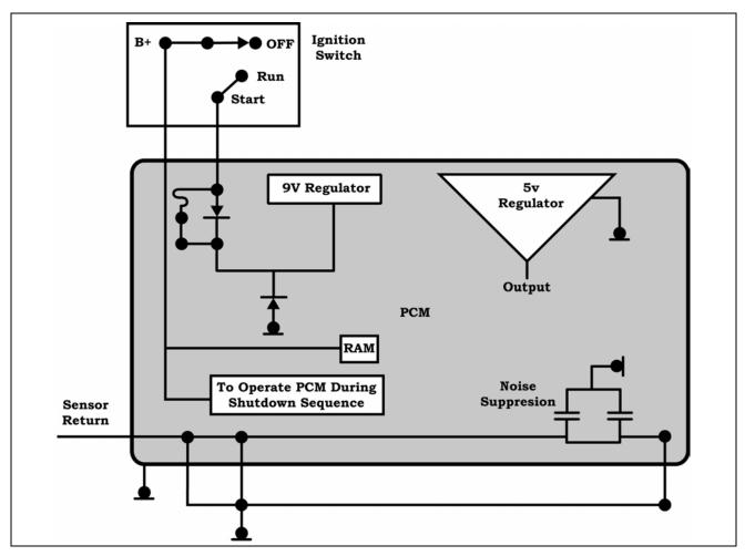
Figure 32 SBEC PCM Power Supplies and Grounds
