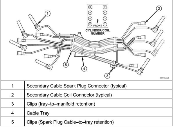
Figure 81 5.7L Spark Plug Cable Routing and Cable Tray
