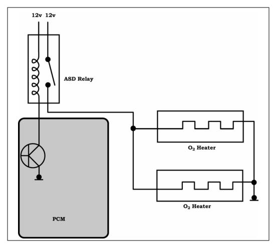
Figure 56 Oxygen Sensor Heater Element - ASD Power / Constant Ground
