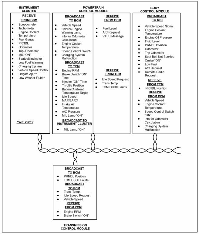
Figure 26 Typical CCD Bus Communication
