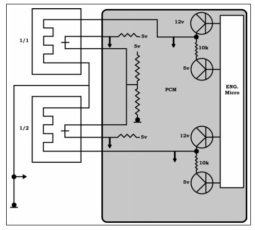
See Figure 55, Page 93 Oxygen Sensor Heater Circuit
