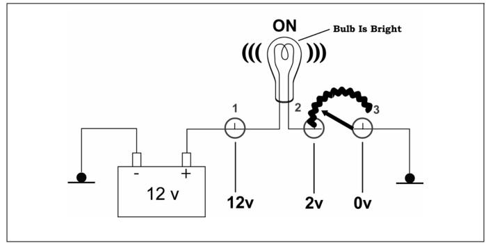
Figure 3 Variable Resistor, Low Ohm Setting
