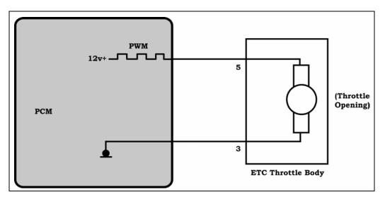
See Figure 96, Page 148 ETC Motor Polarity with Throttle Opening
