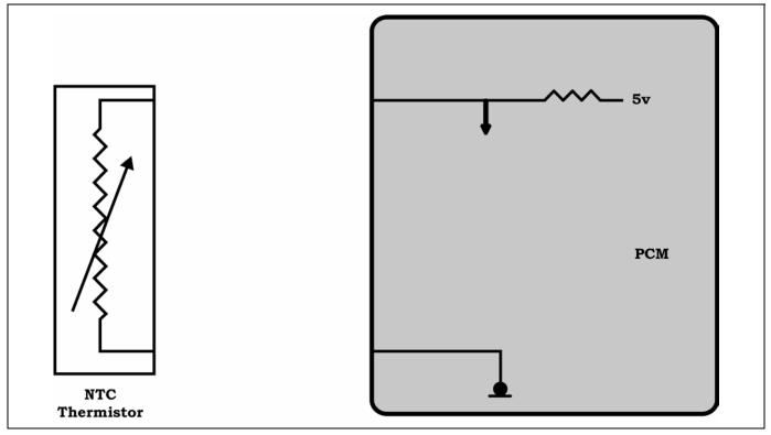
Figure 44 Typical NTC Thermistor Circuit (Completed by Student)
