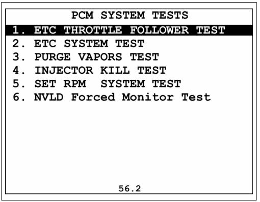
Figure 105 ETC Tests on the DRBIII
