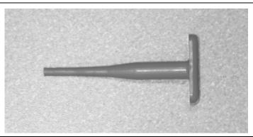
Figure 22 Miller #6934 Pin Removal Tool – JTEC
