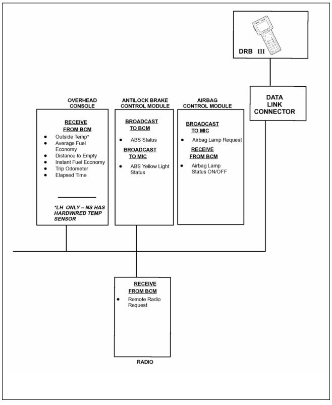
Figure 24 Typical PCI Data Bus Communication
