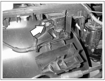
Figure 91 Accelerator Pedal Position Sensors - 2003 5.7L DR
