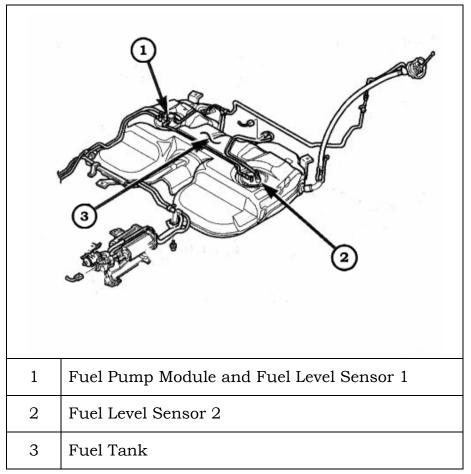
Figure 14 Dual Fuel Level Sending Units on Pacifica (CS)
