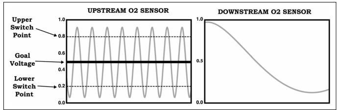
Figure 52 Upstream and Downstream O2 Signal with Efficient Catalyst
