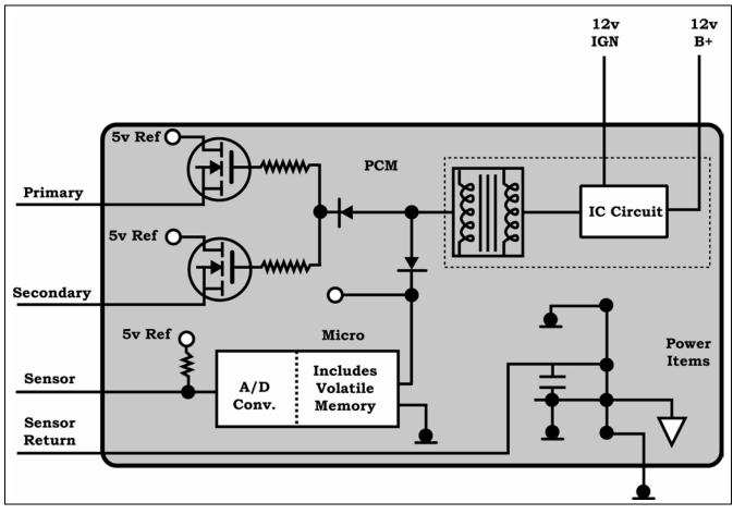
Figure 31 JTEC PCM Power Supplies and Grounds
