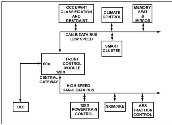
Figure 25 Typical CAN Bus
