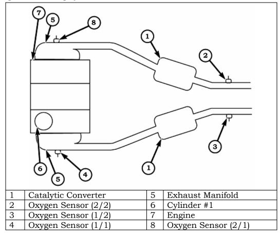
Figure 50 Oxygen Sensor Naming Conventions
