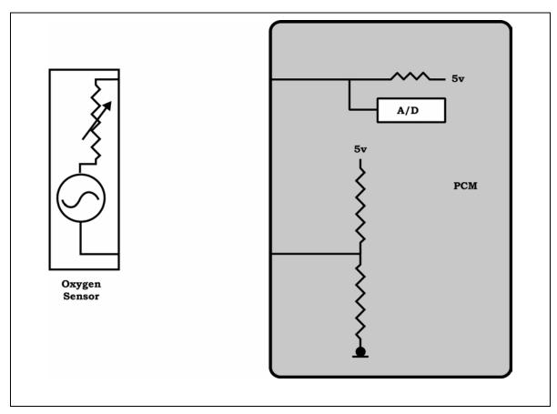
Figure 49 NGC Oxygen Sensor Signal Circuit (Completed by Student)
