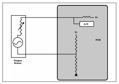
See Figure 49, Page 84 Oxygen Sensor Signal Circuit
