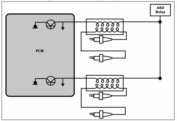
Figure 78 DIS (Waste Spark) Ignition Coil Circuit
