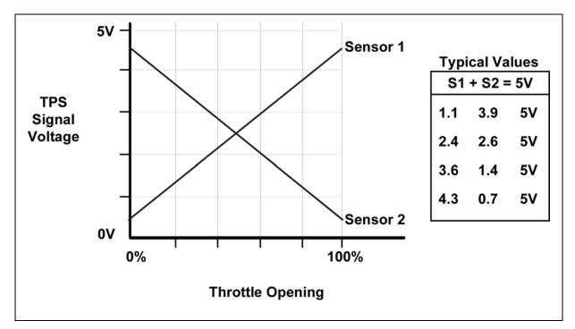
Figure 99 TPS Signal Voltages vs Throttle Plate Position
