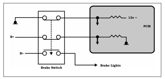
Figure 102 Brake Switch Circuit
