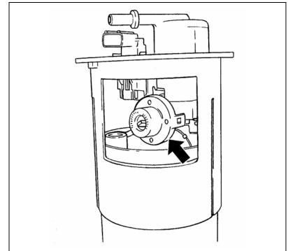
Figure 12 Typical Fuel Filter and Pressure Regulator
