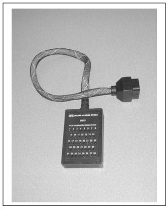
Figure 17 Miller #8815 Pinout Box
