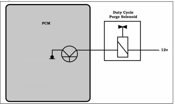
Figure 85 Duty Cycle Purge Solenoid
