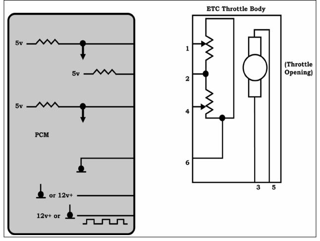
Figure 100 Electronic Throttle Control Circuit (Completed by Student)
