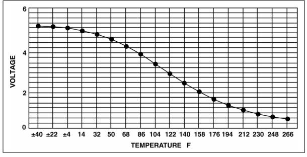
Figure 46 Typical NTC Thermistor Temperature-Voltage Curve
