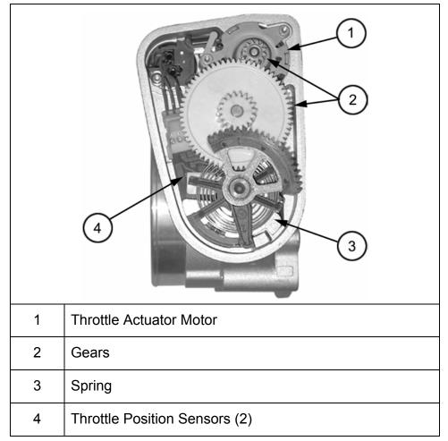
Figure 98 5.7L ETC Throttle Actuator Motor, TPS, Spring and Gears
