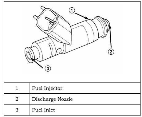
Figure 71 Fuel Injector
