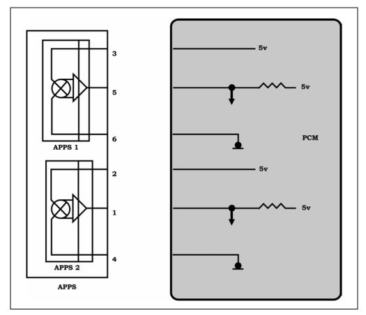
Figure 94 5.7L APPS Circuit (Completed by Student)
