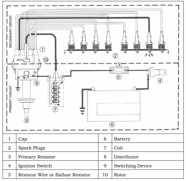
Figure 77 Distributor Type Ignition System
