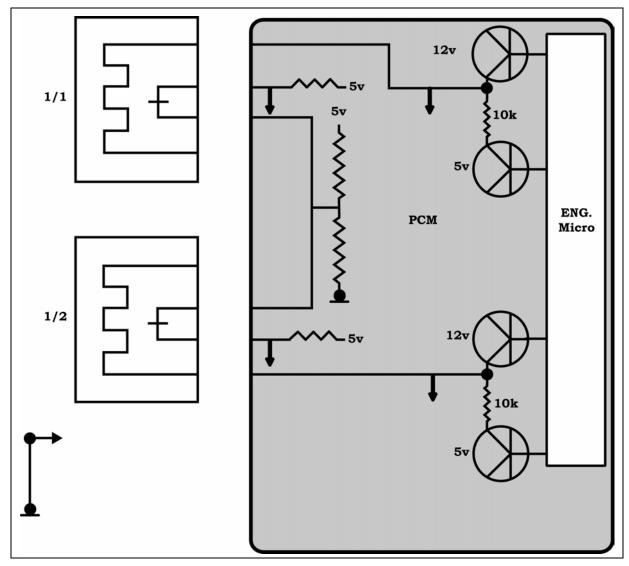
Figure 55 O<sub>2</sub> Sensor Heater Circuits (Completed by Student)
