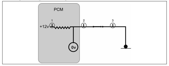
Figure 6 PCM Circuit, Low Input
