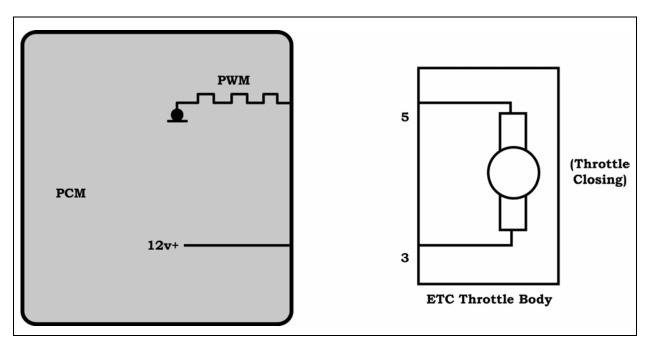
Figure 97 ETC Motor Polarity with Throttle Closing Completed by Student)
