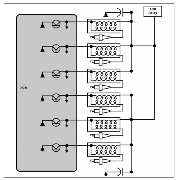
Figure 79 COP Ignition Coil Circuit
