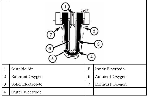
Figure 48 Oxygen Sensor Operation
