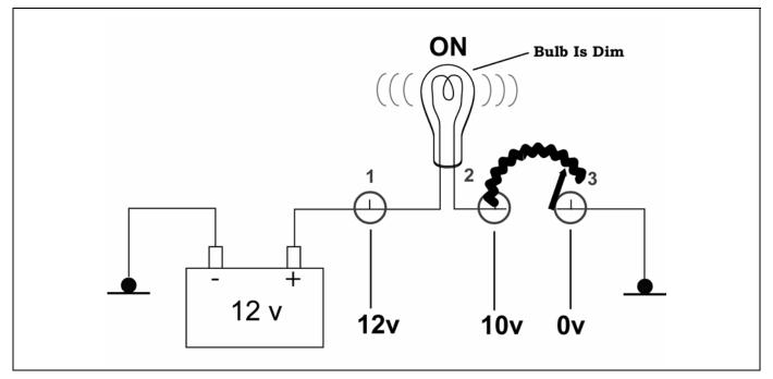
Figure 4 Variable Resistor, High Ohm Setting
