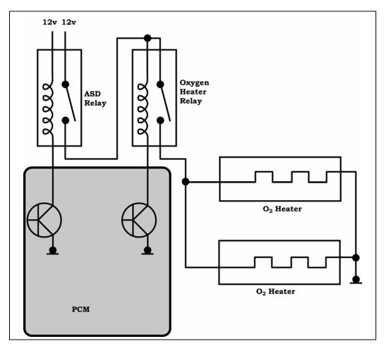
Figure 58 Oxygen Sensor Heater Element - Relay Power / Constant Ground
