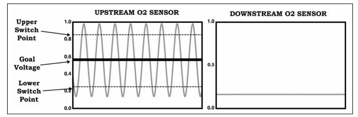
Figure 53 Goal Voltage and Switch Points Shift to Reduce High O<sub>2</sub> Content
