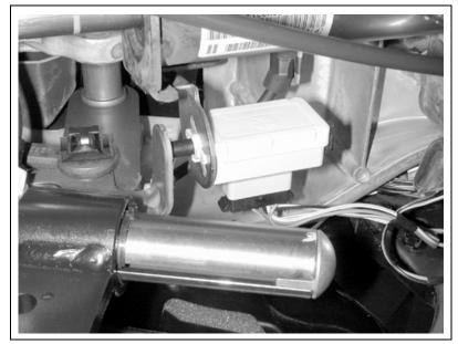
Figure 101 5.7L Brake Switch
