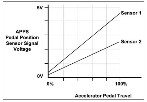
Figure 93 APPS Signal Voltages vs Accelerator Pedal Travel
