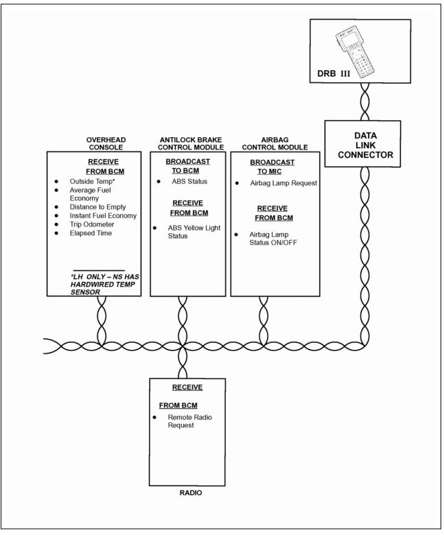
Figure 27 Typical CCD Bus Communication
