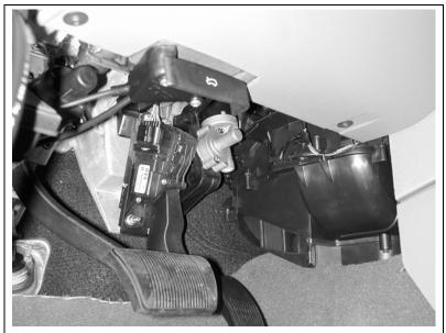
Figure 92 Accelerator Pedal Position Sensors – 2004 HB Durango
