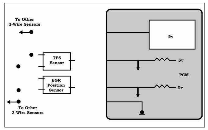
Figure 43 TPS and EGR Position Sensors (Completed by Student)
