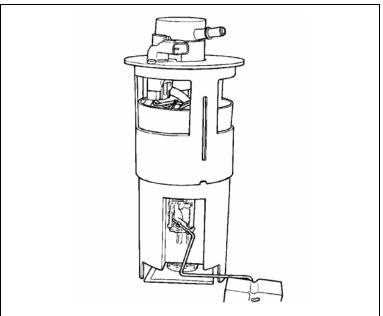
Figure 11 Typical Fuel Pump Module
